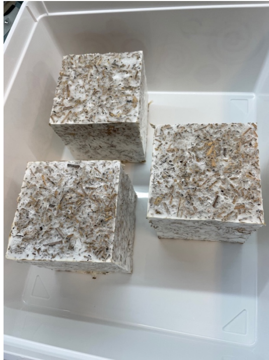
Mycelium blocks in the maturing phase
