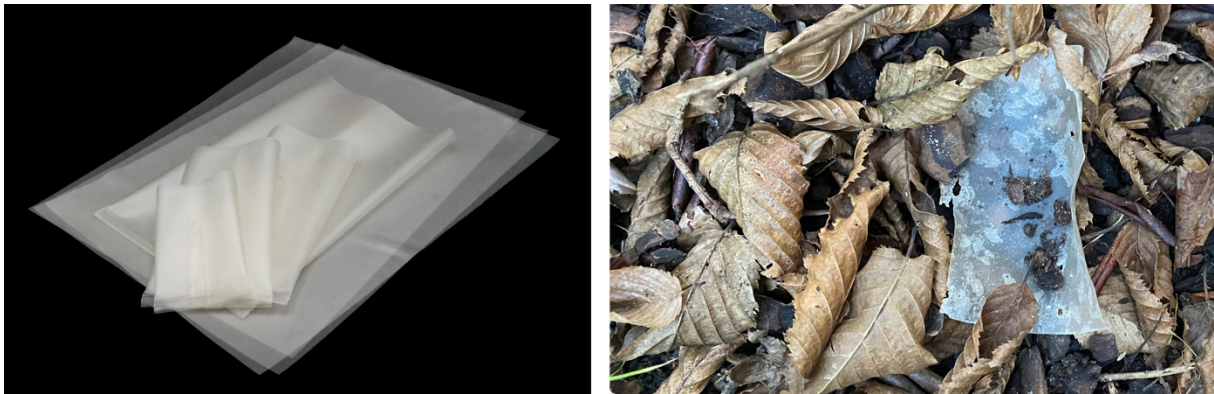
6. l: Meal Bag empty packaging samples and films. r: Meal Bag film weathering process.
